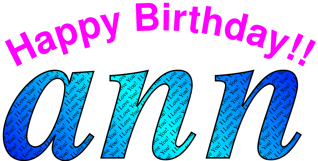
Example 4: Typesetting text on a path, filling character outlines, and using a TeX box as a fill pattern.
